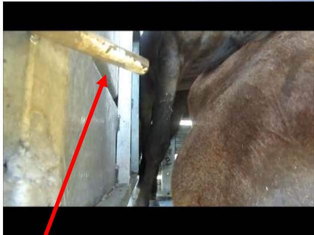
Broken piping inside trailer
