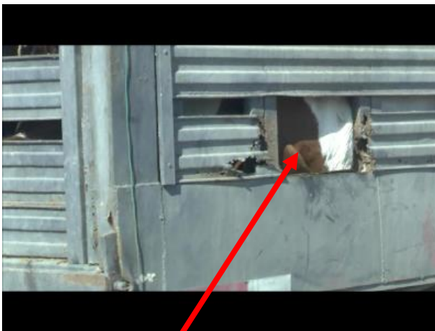
Hole in trailer side – horses' legs can get stuck
