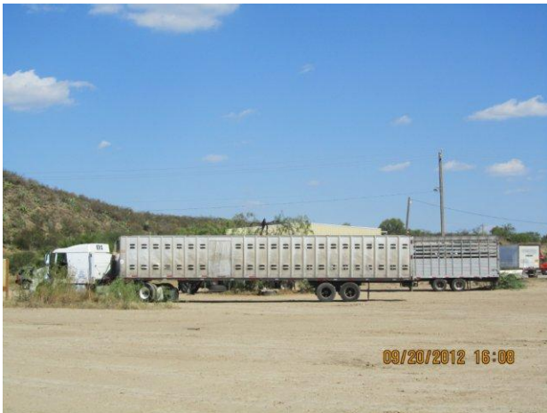
Closed up trailer with insufficient air flow
